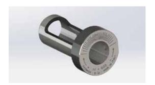
The eccentric bushing for the REV BROACHING TOOL is an essential accessory for any lathe that is not equipped with a Y axis. In fact, this bushing can be used to correct any alignment error that may occur during broaching and slotting.
