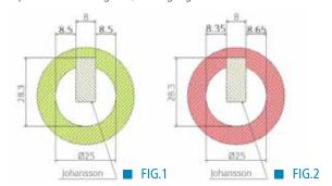
In the example provided in Fig. 1 the measured value 8.50 mm is correct, while in Fig.2 the measured value is 8.35 mm on one side and 8.65 on the other, resulting in an alignment error of 0.15 mm that needs to be corrected.
