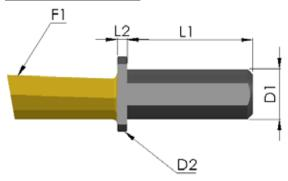
Integral inserts in the MINITOOL line feature a flat side on the collar, with a diameter of 15 mm, allowing the operator to check the correct position of the insert in very restricted amounts of time, through the use of common comparators or gauges. They can be manufactured in two possible alloys: sintered steel or, alternatively, high toughness widia.
